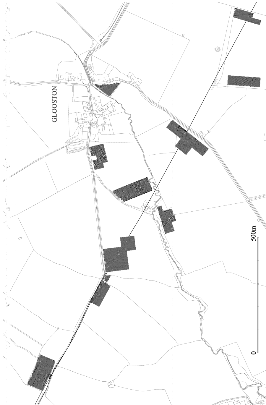
Fig. 7. Geophysical work to date on the Gartree road between Cranoe and Glooston. The dark line shows the projected route of the Roman road.
